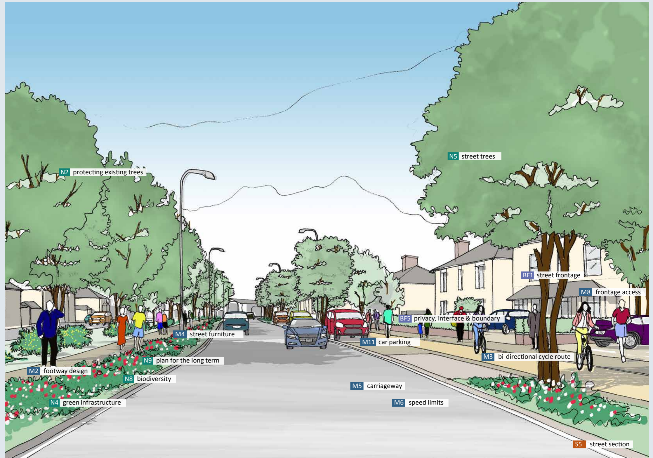
Figure 4.4: Sketch indicating application of the code on the A23 in south Horley including introduction of a bi-directional cycle lane, and planted verges / raingardens.
