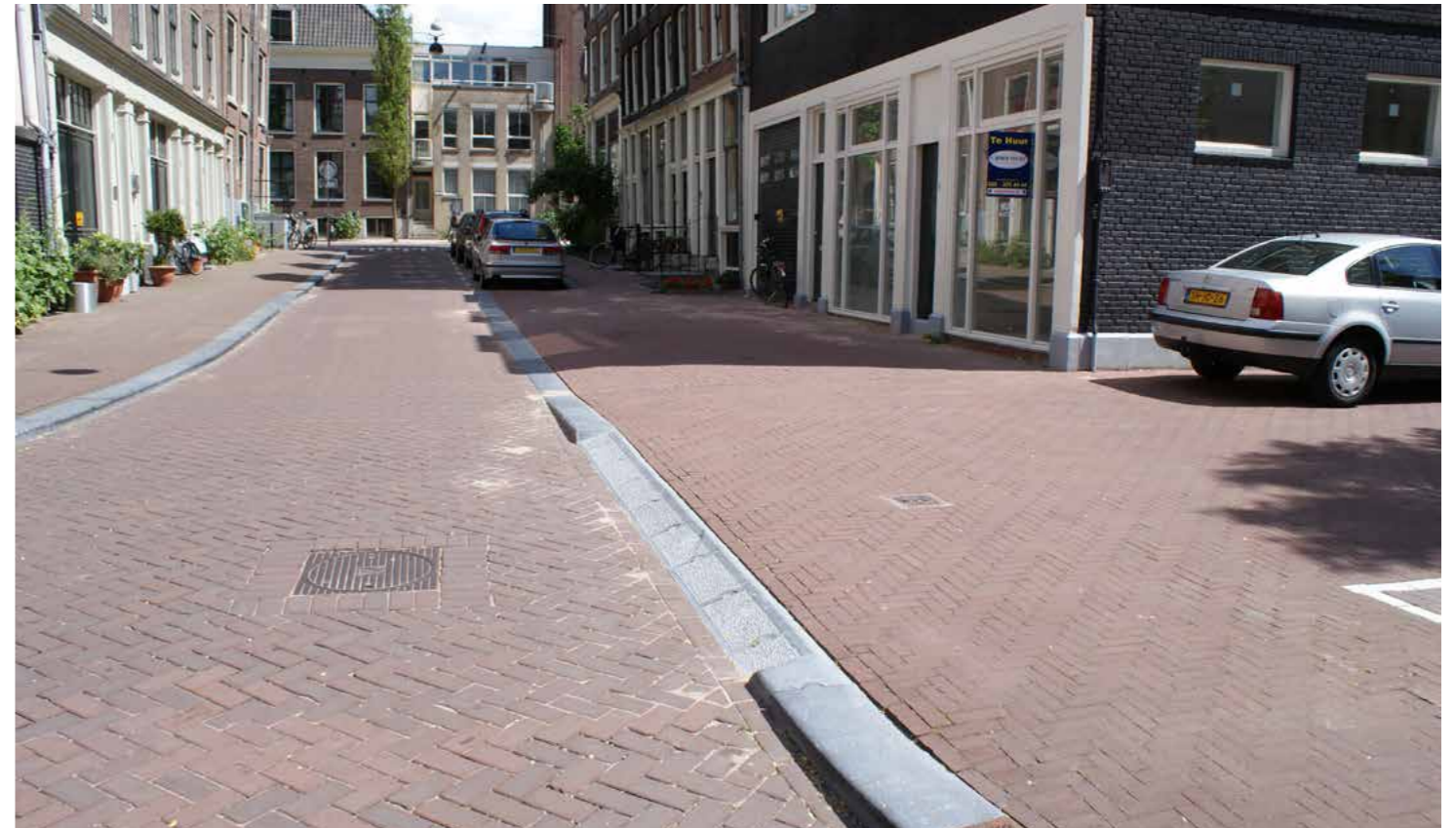
Image 4.4: Example of crossover junction design
