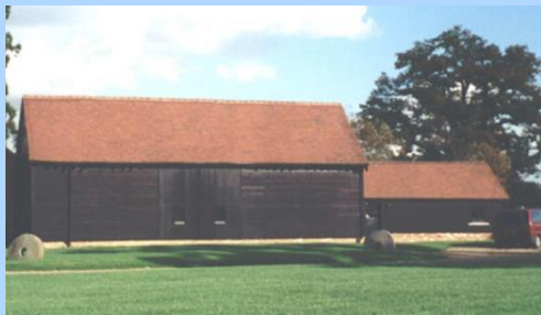
Figure 99: A barn conversion in the borough, showing the general approach of no windows on the public side to maintain the agricultural appearance, including no rooflights, dormers or chimneystacks.
