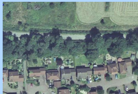
Figure 109: Soft edge to the countryside at Horley with a 15 metre buffer in communal ownership and housing set back 10 metres behind the buffer. Image source: Google maps.
