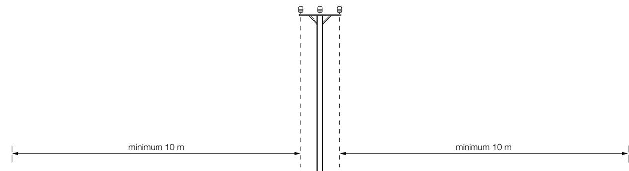
Figure 2 Minimum horizontal distances to overhead power lines
