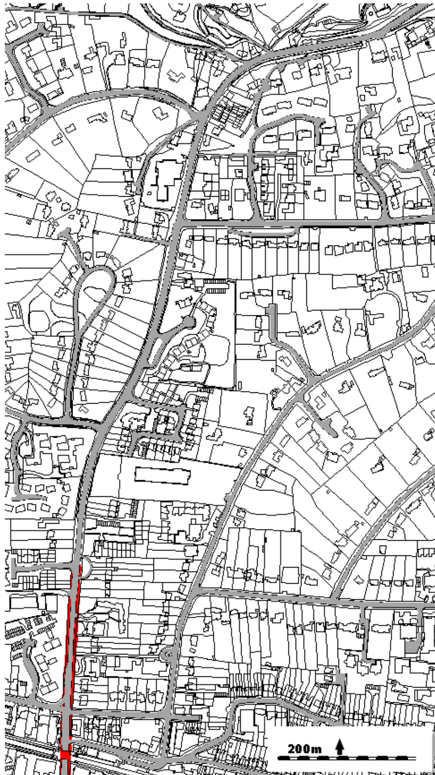
Figure 11: Predicted Exceedences of 40 \mu\text{g}/\text{m}^3 as an Annual Mean Nitrogen Dioxide Concentrations in 2015 on Reigate Hill ( \mu\text{g}/\text{m}^3 )
