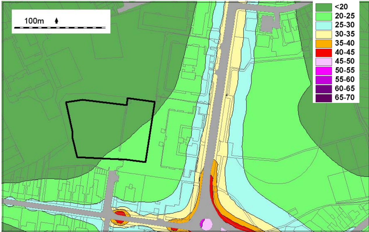
Figure 19: Predicted Annual Mean Nitrogen Dioxide Concentrations Across Area A in 2016 – With Development ( \mu\text{g}/\text{m}^3 )
